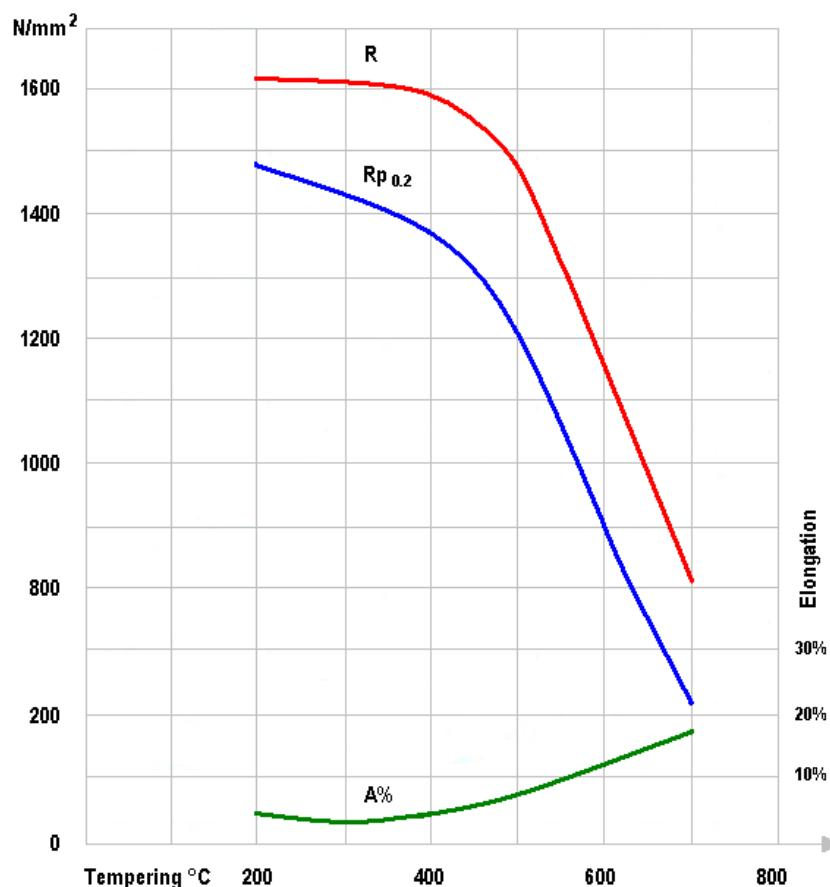
Mechanical testing on rounds of Ø 20 mm after quenching at 1050°C in oil
